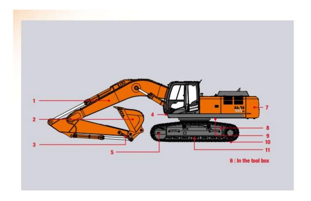
1 Reinforced thick steel front section. (H-boom / H-arm) Thicker steel arm end. Damage prevention plate and square bars.
